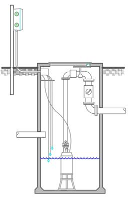
Pump w/ Stand Typically used in condensate and leachale transfer applications. Stand places pump inlet above sediment. Disconnect methods allow easy access without entering wet well
