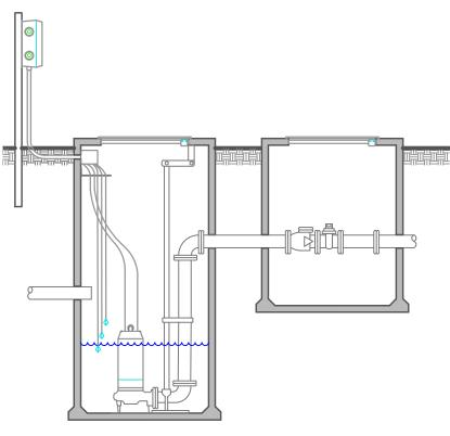
**Guide Rail** Typically used in waste water applications w/ large solids separate valve box recommended
